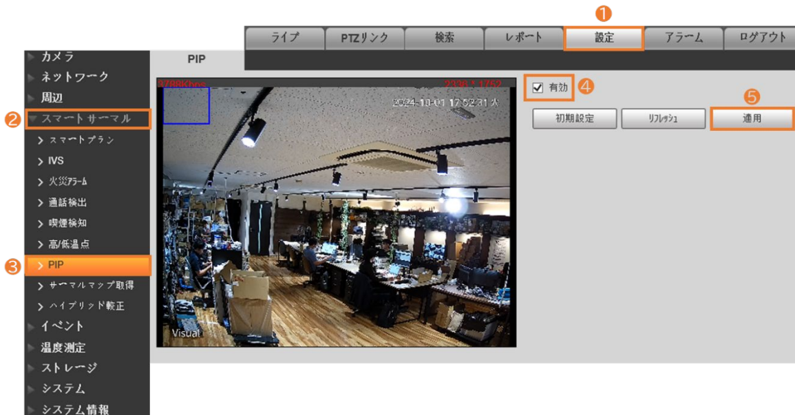
図5-52 PIP(Pic in Pic)
